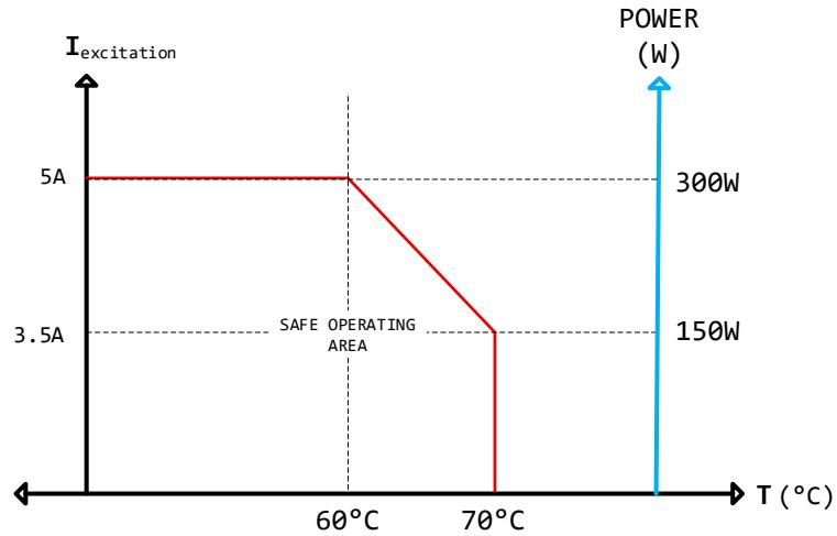
DAVR90 can deliver full 300W power into the excitation winding under continuous operating conditions up to 60°C ambient temperature limit. Above this temperature level, continuous excitation power is derated according to the SOA graphic given above. From 60°C to 70°C ambient conditions, excitation power must be derated by -5%/°C linearly up to 70°C, which is the maximum operating temperature limit of the AVR unit.
