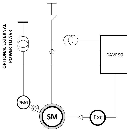
The power to AVR can be connected in various ways, including an external isolated power supply with correct specifications. The system can also be connected in SHUNT or AUXILIARY power supply modes or can be fed directly from a PMG alternator. If an external AC source is connected, ensure correct voltage and isolation limits for safe operation.
