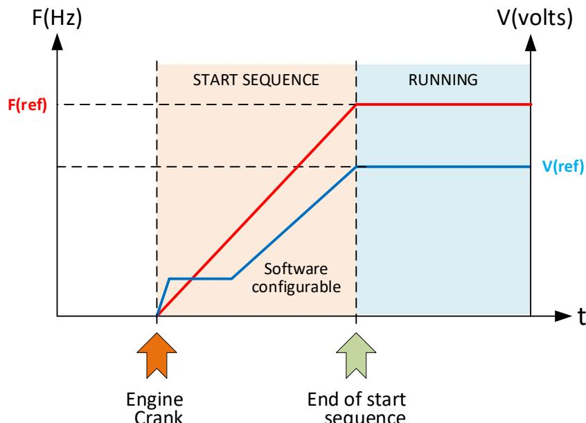
As graphically shown above, the START SEQUENCE of the AVR must be configured to suit the required application. The sequence starts with the engine cranking and ends with the user determined condition, where normal AVR mode
