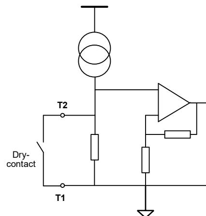
[T1-T2] and [T3-T4] can be set as mixed signal inputs, any number can be set as temperature inputs while remaining of the three inputs can be set as digital inputs at the same time.
