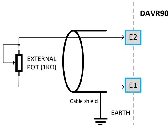
If the cable length exceeds 1m, it is recommended that a shielded cable is used, and the cable shield is connected to EARTH terminal near the AVR side only, opposite end of the shield should be left unconnected. DAVR90 detects the external POT connection status and user is required to set the “External Pot Effective Range” parameter [P142] to suit their application, as shown in table below:
