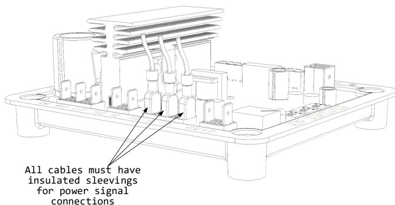
All power connection terminals MUST be connected, using insulated sleeving cable terminals. AUX terminals and communication sockets are galvanically isolated from the power terminals, but precaution must be taken during application to make sure that insulation levels are not exceeded.
