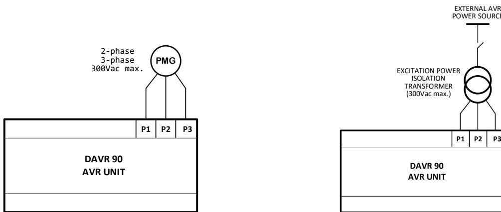
All “Power and Sense” input terminals are galvanically isolated from the “Auxiliary & Communication” signal terminals, and the isolation is rated at 500Vac.
