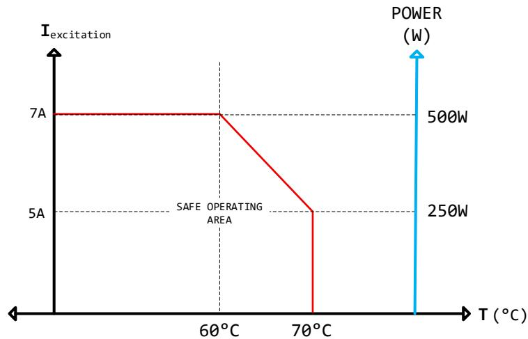
DAVR100 can deliver full 500W power into the excitation winding under continuous operating conditions up to 60°C ambient temperature limit. Above this temperature level, continuous excitation power is derated according to the SOA graphic given above. From 60°C to 70°C ambient conditions, excitation power must be derated by -5%/°C linearly up to 70°C, which is the maximum operating temperature limit of the AVR unit.
