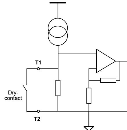
[T1-T2], [T3-T4] and [T5-T6] can be set as mixed signal inputs, any number can be set as temperature inputs while remaining of the three inputs can be set as digital inputs at the same time.
