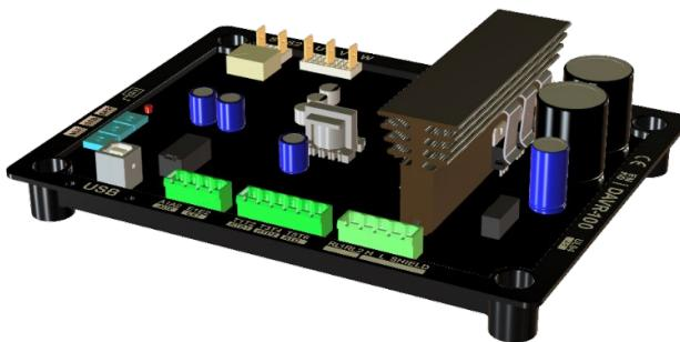
Based on the digital control architecture, DAVR100 regulates the stator voltage using precise RMS calculations, considering all distortions on the voltage waveforms, which results in exceptional performance.
