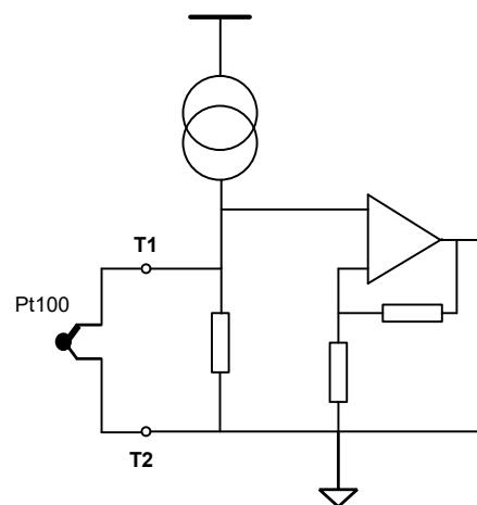
All temperature measurement inputs have the block schematic as shown in the figure above. The "equipotential" ground connection is common to all AUX signal input hardware and therefore, when connecting temperature sensors and external control equipment, care must be taken to ensure safe operation.
