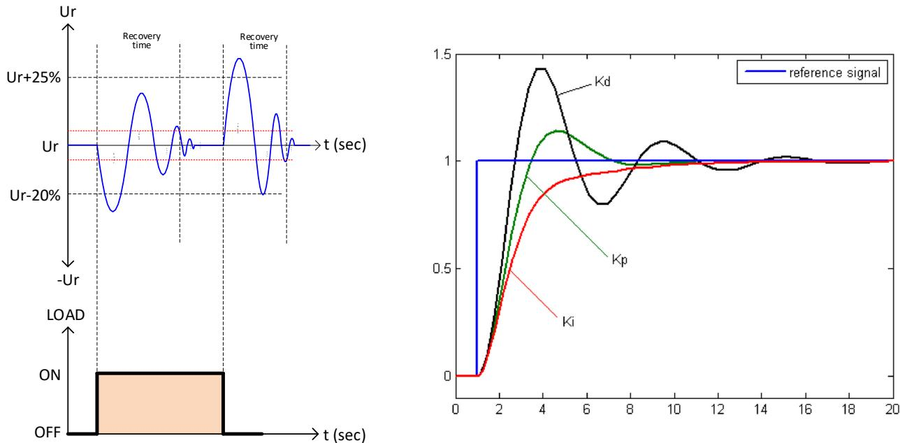
The limits of the recovery time and the transient response levels are determined by ISO8528-5:2018 and user should set AVR PID and LAM parameters to ensure that overall generator can perform according to the required “G” class operational limits.
