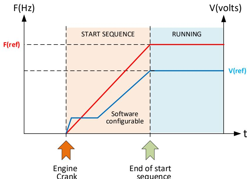
As graphically shown above, the START SEQUENCE of the AVR must be configured to suit the required application. The sequence starts with the engine cranking and ends with the user determined condition, where normal AVR mode
