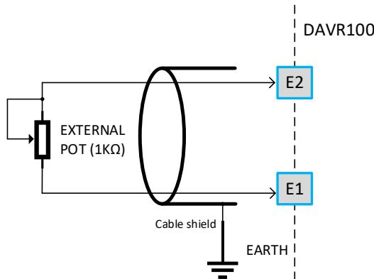
If the cable length exceeds 1m, it is recommended that a shielded cable is used, and the cable shield is connected to EARTH terminal near the AVR side only, opposite end of the shield should be left unconnected. DAVR100 detects the external POT connection status and user is required to set the “External Pot Effective Range” parameter [P142] to suit their application, as shown in table below:
