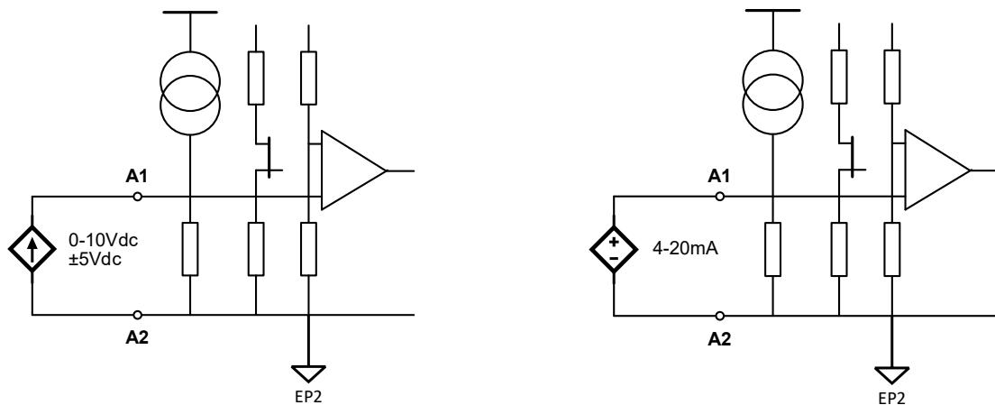
Analogue input signal connection can be arranged as:
