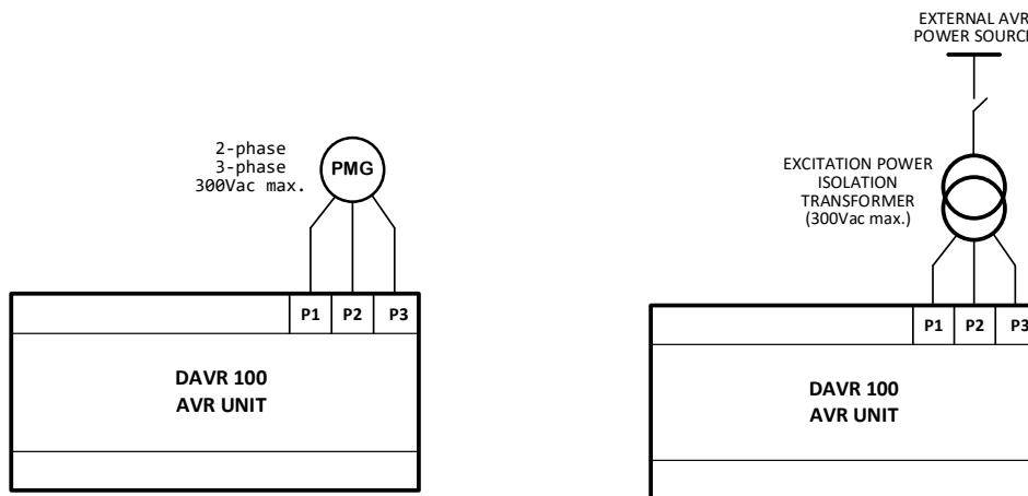
All “Power and Sense” input terminals are galvanically isolated from the “Auxiliary & Communication” signal terminals, and the isolation is rated at 500Vac.
