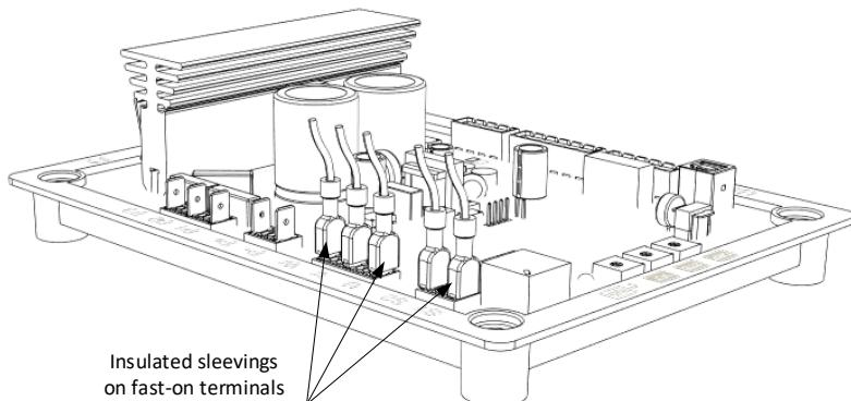
All power connection terminals **MUST** be connected, using insulated sleeving cable terminals. AUX terminals and communication sockets are galvanically isolated from the power terminals, but precaution must be taken during application to make sure that insulation levels are not exceeded.
