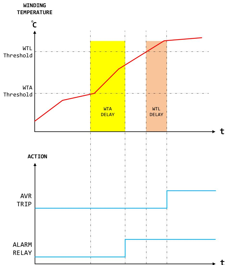
**NOTE:** This “**Cascade Protection**” application can only be applied if the AVR is fed from PMG power unit. This application is not valid for SHUNT and/or AUXILIARY power connections.
