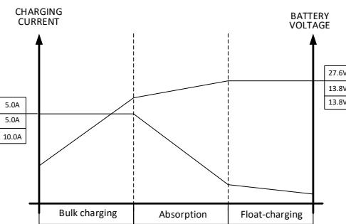
During BULK stage, battery is depleted, and terminal voltage is low, and charger delivers full rated current into the battery. During this phase, battery terminal starts to rise.
