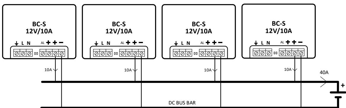
In the example given above, total battery charging current is 40A and maximum allowed cable size for charger terminals is  $1.5\text{mm}^2$  therefore, daisy-chain wiring of the chargers is not a good practice as the current density across the wire will accumulatively increase to 40A, which the wire cannot carry.
