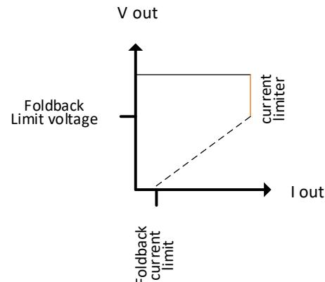
During foldback current limit state, the charger dissipates a very small power, hence allowing a long-term reliable charging lifetime for the system.
