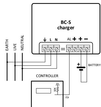
An internal pull-up resistor may be required, depending on the control unit's input hardware configuration.
