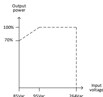
Input power derating also changes with the operating environment temperature, and this must be taken into account, when calculating maximum available output power from the charger at any given operating conditions.
