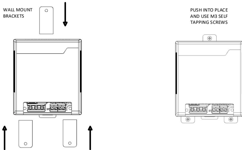
*For wall mounting, use the wall-mount brackets (optional) and slide the brackets into their place on the back side of the charger enclosure. Use M3 self-tapping steel screws to fix the charger onto the mounting surface. First install the bottom brackets, fix the charger on the wall, then fix the top bracket. Ensure that; the charger is fixed securely on the wall and in vertical position.*
