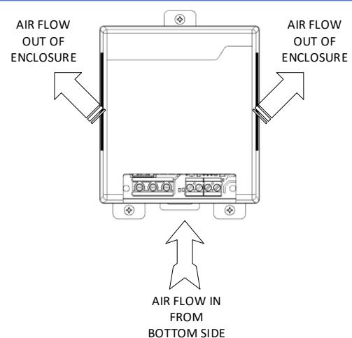
There are no very hot surfaces on the charger enclosure, since the heatsink is mounted inside the plastic case.
