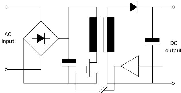
Incoming mains power is rectified and used as DC source for the switching power stage. A high frequency transformer is used to provide galvanic insulation between the mains input and DC output.
