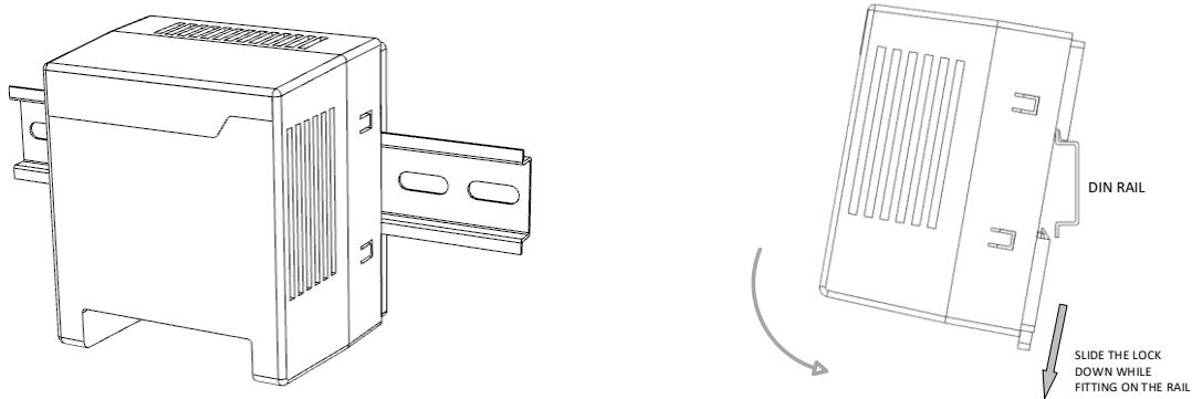
*Ensure to pull the rail lock down with a suitable screwdriver before placing the unit on the DIN rail, then release the lock and ensure that it grips the rail tightly.*
