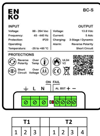
BOOST function will stay active, as long as the BOOST control terminal is connected to battery +ve terminal-potential. Therefore, BOOST duration must be controlled with an external control unit.
