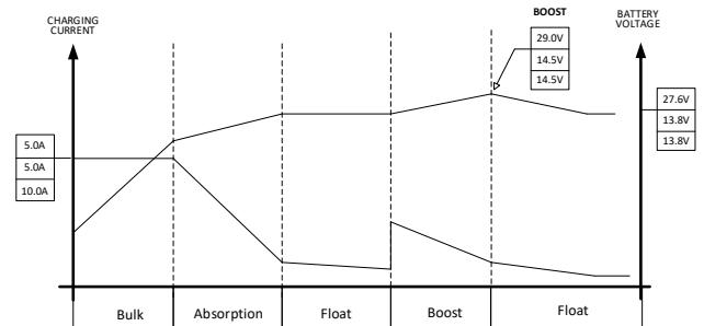
BOOST charging function must be controlled with an external control device, such that, activation repetition period and active duration should be set to keep battery health at its top state.
