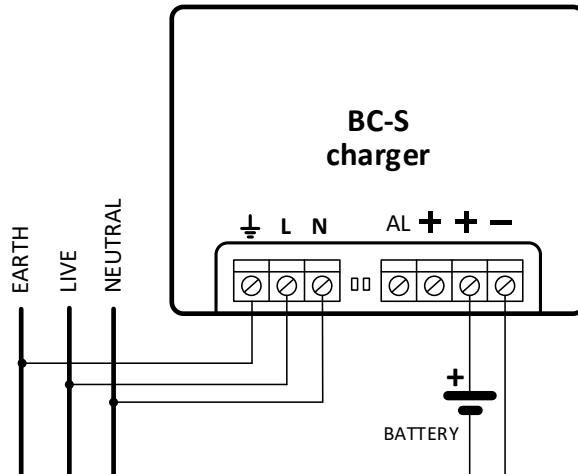
CHECK BATTERY TERMINAL VOLTAGE VALUE AND MAKE SURE THAT, YOUR CHARGER HAS THE CORRECT VOLTAGE RATING TO MATCH YOUR BATTERY. REFER TO THE TERMINAL DESCRIPTION AND WIRE GAUGE TABLE BEFORE ATTEMPTING TO CONNECT WIRES TO YOUR CHARGER.
