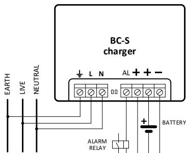
If ALARM function is going to be used with a control unit, then there is no requirement for an external relay. Please refer to the connection diagram below:
